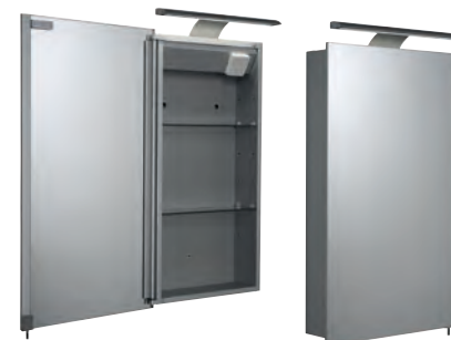
Jefferson Single Door LED Illuminated Cabinet ■ 700 x 400 x 120mm ■ Aluminium cabinet with double sided mirrored door ■ Decorative LED lighting bar with rocker switch operation ■ Integrated shaver socket ■ Two adjustable tempered glass shelves ■ 180 Degree hinges for increased accessibility ■ Easy install Hang 'n' Lock™ system ■ IP44 Rated, suitable for use in the outside zone 103.WC147769E £437
